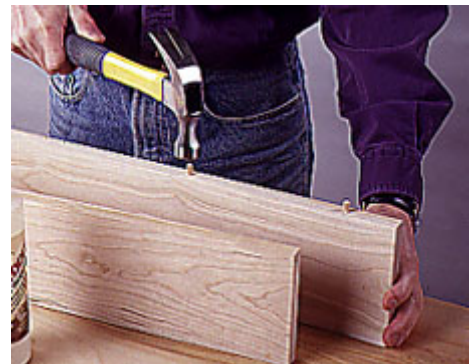
4 -Once the holes are bored, spread glue in the holes and along the board edges. Then gently tap the dowels into place.
