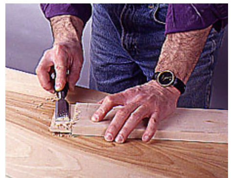
10 -Use a sharp chisel to remove the saw marks on the cheeks and to cut the tenon to the finished dimension.
