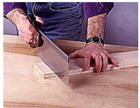
9 -Once the cheek cuts are made, lay the board flat and make the shoulder cuts. Again, stay on the waste side of the line.
