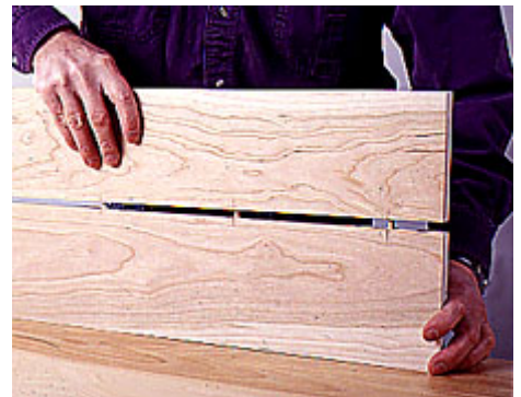
5 -Position the mating board so its holes align with the dowels in the first board. Then squeeze the two boards together.
