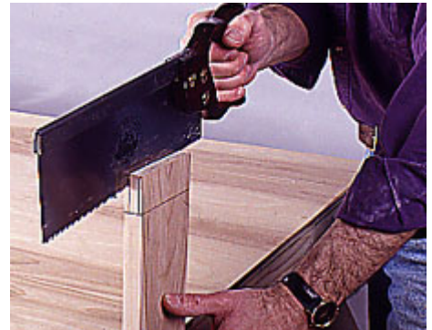
8 -Clamp the board upright and use a backsaw to cut along the layout lines. Be sure to cut on the waste side of the line.
