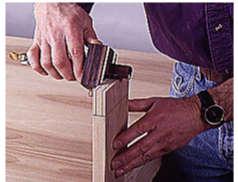
7 -Use a marking gauge to mark the tenon lines on the edges and the end of the board. Center the tenon on the end of the board.
