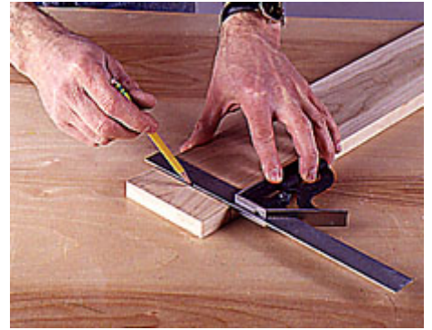
6 -Begin laying out a tenon by marking a shoulder line on all four sides of the board. Use a square and a sharp pencil.
